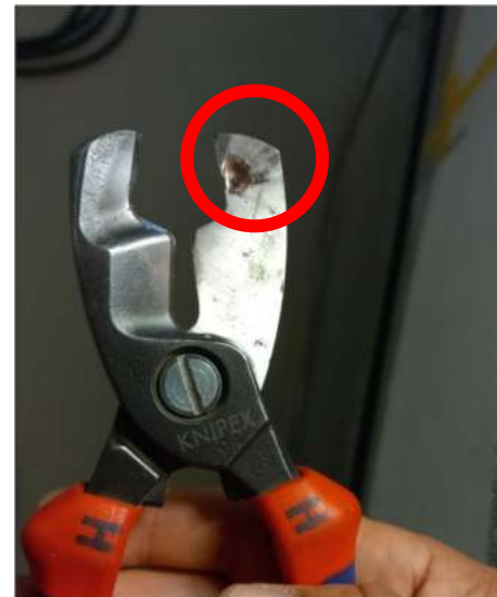
Pliers (impact of the electrical arc)
